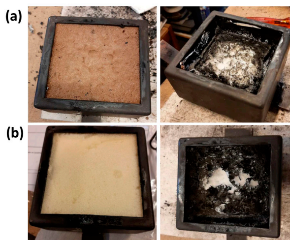
Figure 7. (a) bio-based RPUF and (b) RPUF-conv before (left) and after (right) burn.
